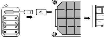
3 LED stops blinking and turns on when the batteries are fully charged
