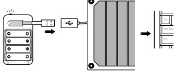
3 LED stops blinking and turns on when the batteries are fully charged.
