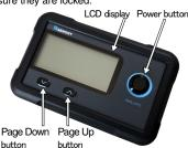
2 Press the Power button on the monitoring screen to activate the battery. The backlight will then be lit and the LCD Display will show the present voltage.
