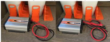
2 Connect the input cable of the inverter and battery cable of the charge controller with positive terminal of the built-in battery of VS12-B115LAV battery compartment. Then . connect input & output cable of this product with positive terminal of the built-in battery. Attach both terminal covers
