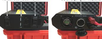
3 To power appliances with DC12V input outdoors, connect the DC12V Output Cables to dust and water proof connectors and the processed end to the appliances.
