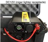
3 To power appliances with DC12V input outdoors, connect the DC12V Output Cables to dust and water proof connectors and the processed end to the appliances.
